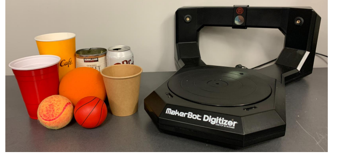
Fig. 4: Real-world objects (tin cans, foam balls, and paper cups) of various sizes (left) and the MakerBot Digitizer 3D scanner (right).
